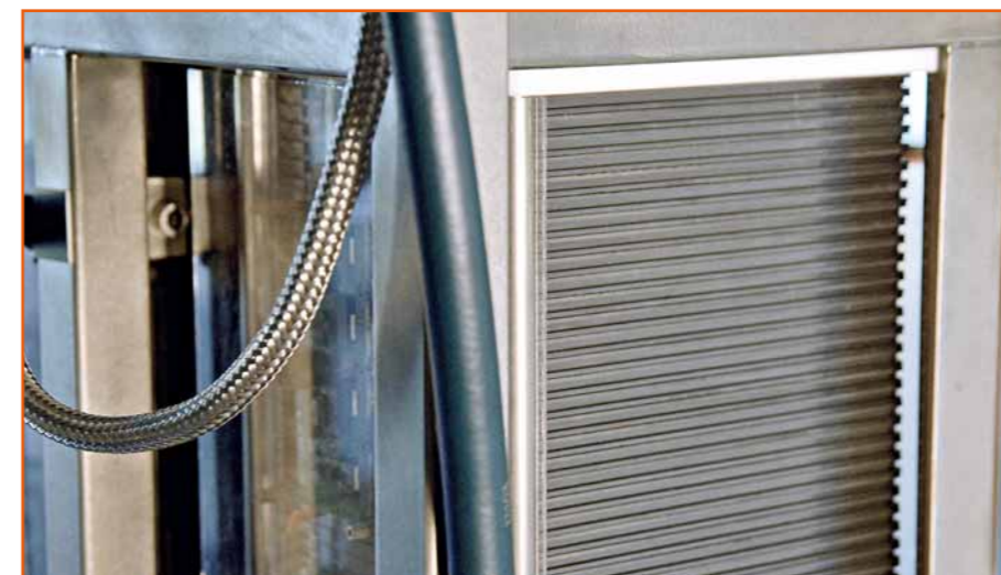
Experimental fuel cell stack: the detailed view shows how closely together the individual cells are packed
