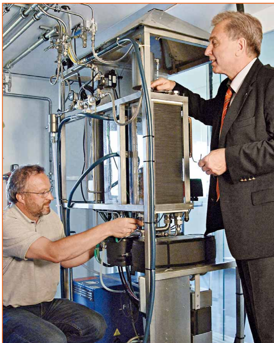
Airbus specialists examine the operating parameters of fuel cells on a test-rig under controlled laboratory conditions
